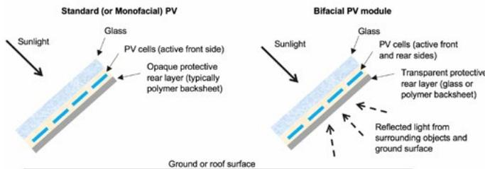
Figure 1.1: Schematic showing basic differences between monofacial and bifacial modules
