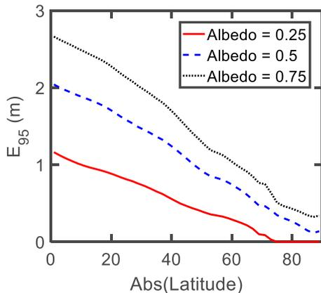
Figure 3.1: Average minimum elevation (E95), or height, to achieve 95% of the maximum energy production as a function of latitude at a fixed ground albedo (Xingshu Sun)
