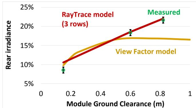
Figure 2.7: Comparison of RayTrace (Radiance) and VF models for 3-row mock array, using 2 months of field data (Deline, 2017)
