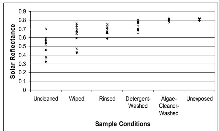
Figure 2.12: Effect of soiling on roofing surface albedo values. Cleaning process was cumulative: dry wiping, rinsing with water, washing with detergent, and washing with algae cleaners. (H. Akbari)
