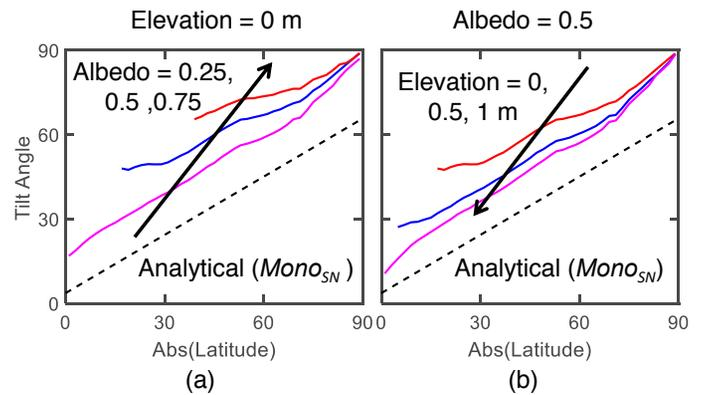
Figure 3.2: Optimum tilt angles for a range of albedos and latitudes (Xingshu Sun)
