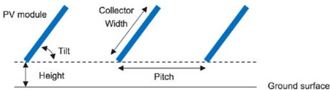
Figure 2.3: Geometrical factors impacting amount of light to module back surfaces
