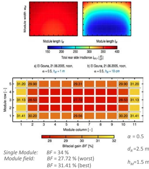
Figure 2.10: Simulations showing variation in irradiance across a single module, and variations in Bifacial Gain across an entire array (J. Libal, 2017)
