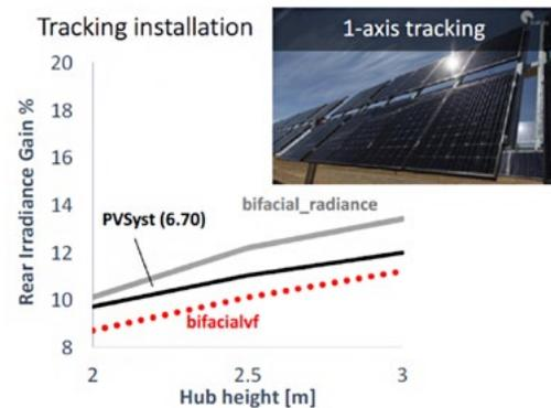
Figure 2.5: Single axis tracking simulations for 2x portrait configuration, 0.35 GCR, 0.3 albedo (gtm Webinar, 2018)
