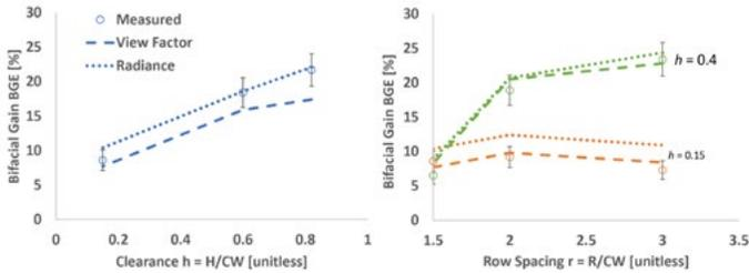
Figure 2.6: Fixed tilt simulations compared against a 3-row test bed in Golden, Colorado (Palaez, 2018)
