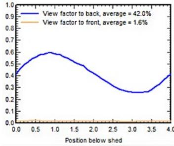
Figure 2.2: Average View Factor for the entire back surface of the PV module, for each ground surface point. Simulation run with PVsyst 6.7.2, Tilt 30°, Pitch 4m, Shed width 2m, Height 1m, albedo 30%, Raleigh, NC.
