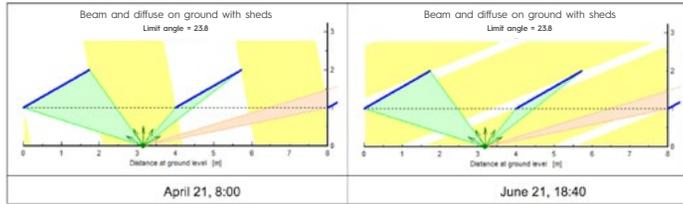
Figure 2.1: The View Factor (fraction of light received on the module back surfaces) is the same for each ground surface point regardless of time of day or time of year (PVsyst)
