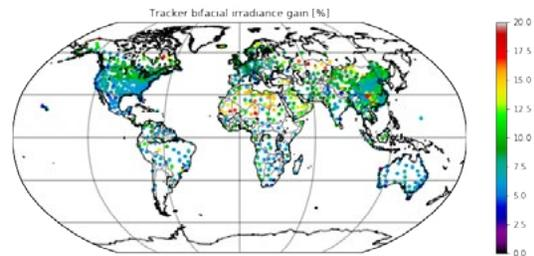
Figure 3.3: Modeled bifacial irradiance gains: 1-axis tracking, 2x portrait, 0.35 GCR, 0% shading and mismatch, natural ground cover albedo from NASA, h = 3 m (local albedo may be under-reported by satellite imagery) (gtm Webinar, 2018)
