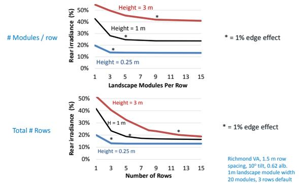
Figure 2.8: Illustration of edge effects in bifacial system modeling (Deline, 2017)
