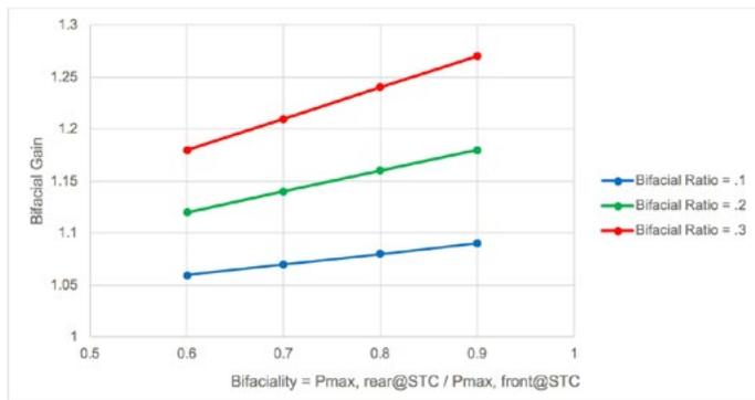
Figure 1.2: Impact of Bifaciality and Bifacial Ratio on Bifacial Gain
