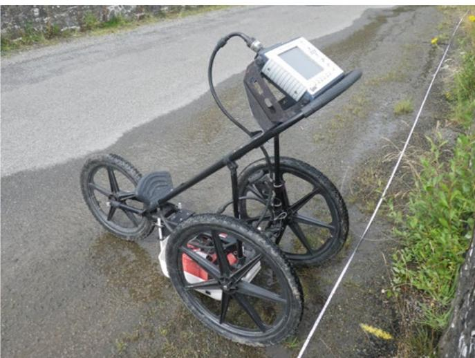
Figure 1: GPR trolley used to push antenna over road surface
