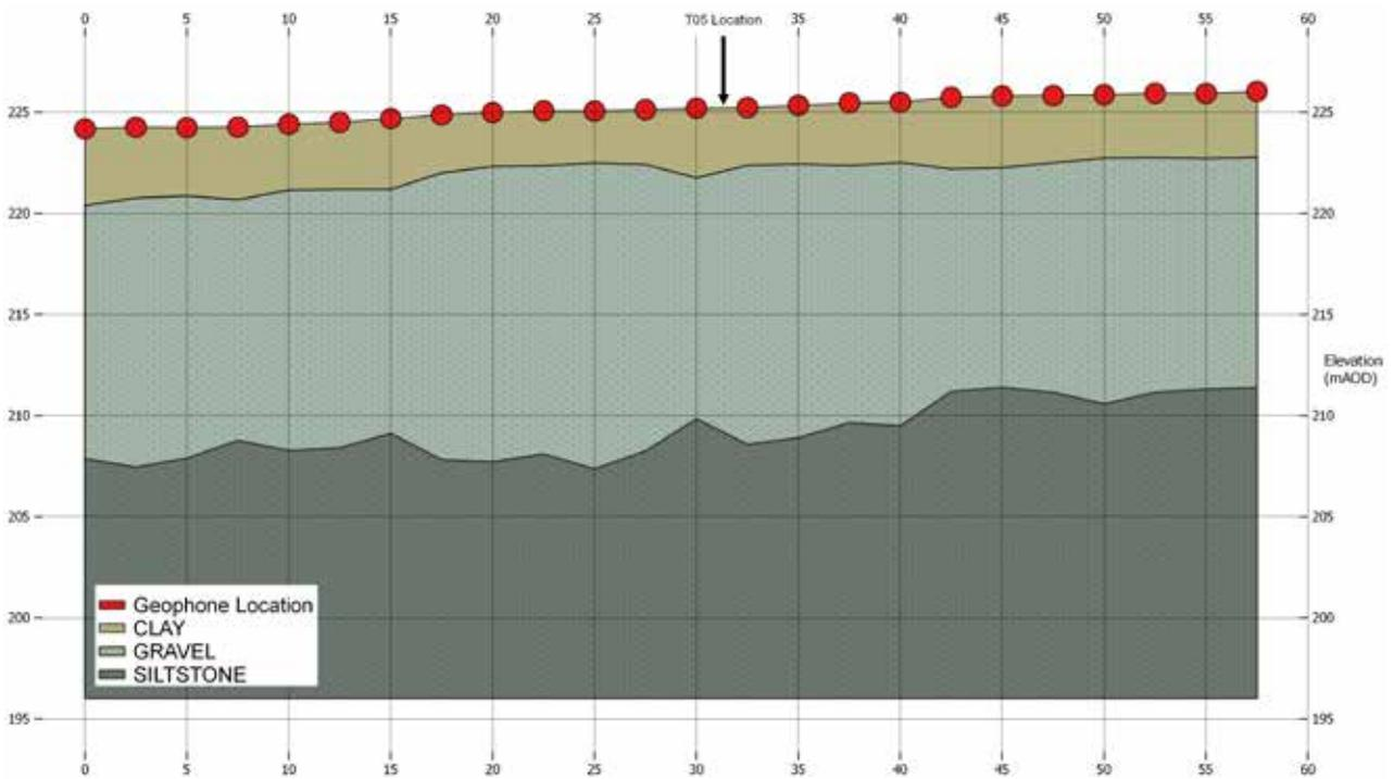
Seismic refraction ground profile (A-B)
