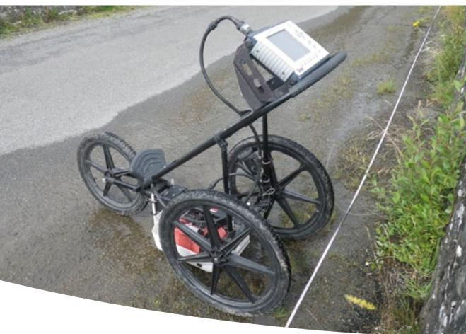
Figure 1: GPR trolley used to push antenna over road surface
