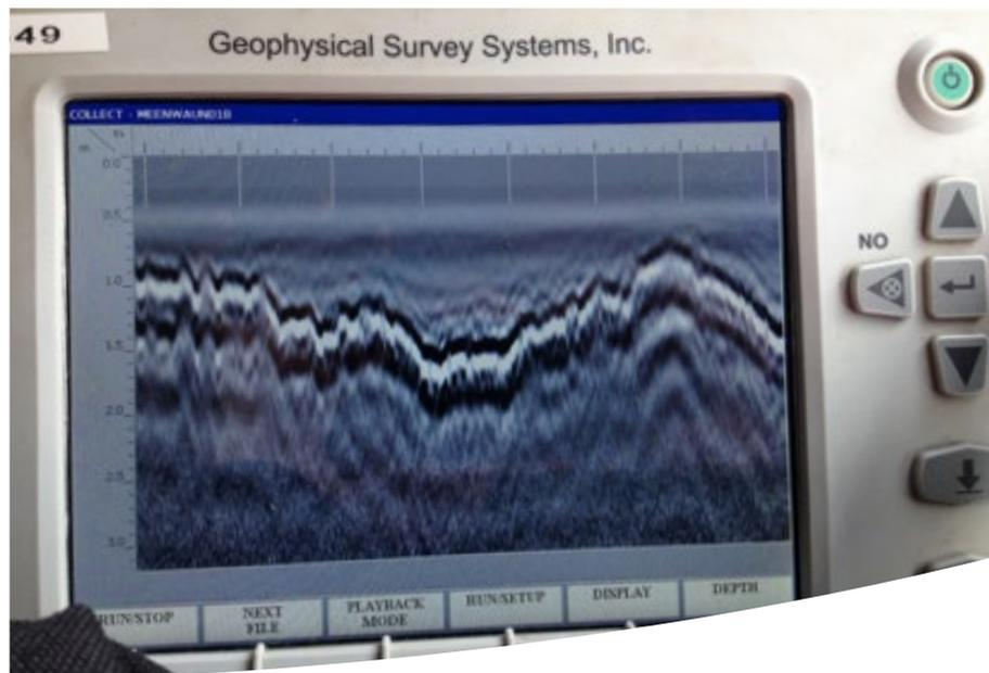
Figure 2: GSSI controller 3000 display screen during data acquisition
