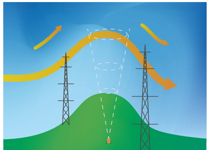
Complex airflow over a hill where any measurement taken will differ from location to location - either an averaged volume measurement, or two independent single point measurements
